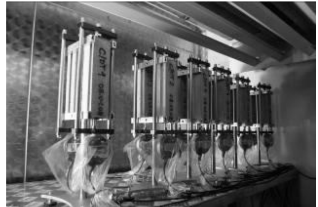
Figure 1. Apparatus for the measurement of length change of hardened concrete according to ASTM C490-86 placed in a climatic chamber.
